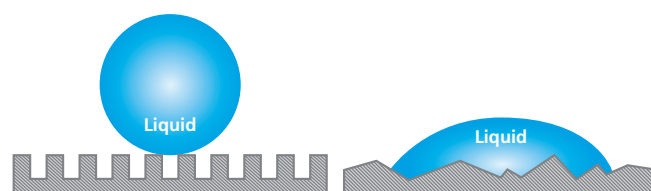
Figure 3 Droplet on (a) Cassie-Baxter (b) Wenzel state
